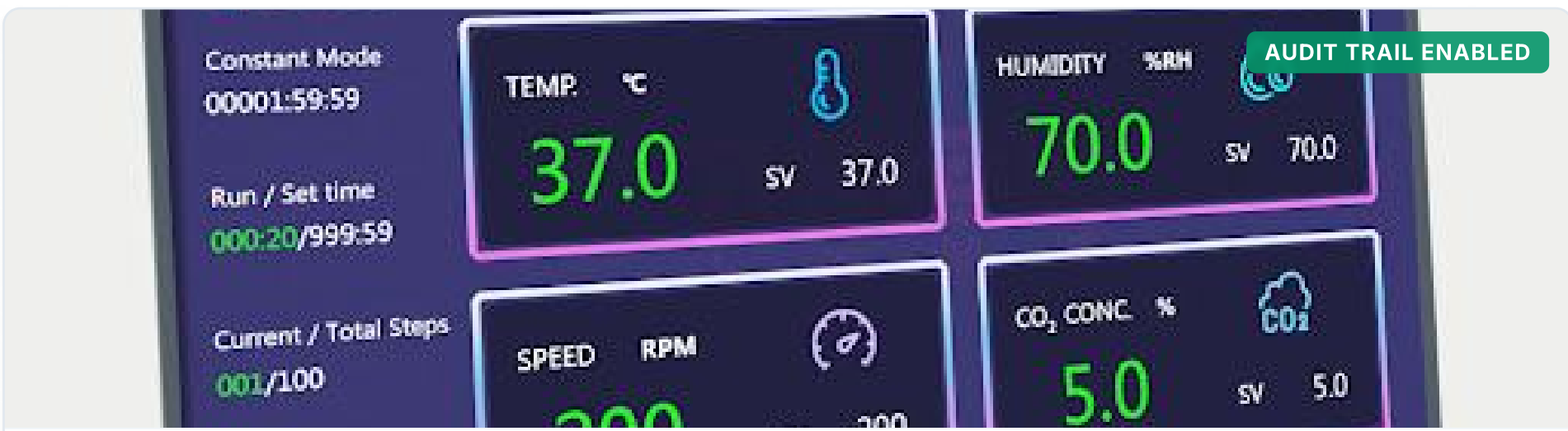
Fig. 1: Continuous multi-parameter display, run/set times, and non-volatile operational status
