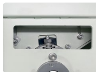
Stepless Adjustable Shaking Diameter
