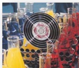
Forced Air Convection Delivers Excellent Temperature Uniformity
